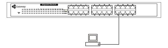
The Link/Act LEDs for each UTP port light green when the port is connected to a Gigabit Ethernet, Fast Ethernet, or Ethernet station. If the indicator is blinking green, data is being transmitted or received.
